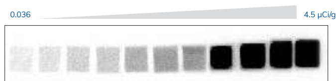
Figure 1. American Radiolabeled Chemicals Carbon-14 standard exposed to Storage Phosphor Screen for three hours then imaged on the Sapphire Biomolecular Imager.
