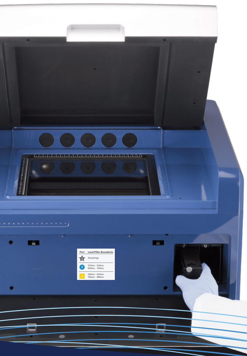
A. Remove optical module from system. B. Remove and replace filter. C. Load new laser and filter combination into the system.
