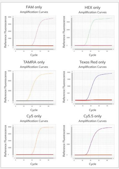
Multiplex qPCR reaction were scanned for all 6 channels in an Azure Cielo Dx Real-Time PCR system. Single channel amplification curves were as expected, with no signal leakage or crosstalk.
