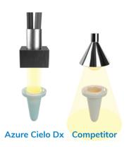
Single illumination light sources can deliver light both in and out of the wells, resulting in higher background, and less light hitting the sample. Azure Cielo Dx uses fiber optics to directly deliver light to each indivdual well.
