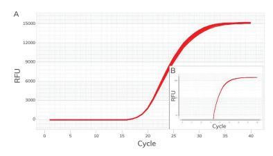
Unparalleled uniformity. Amplification curves for 96 replicates shown on a linear plot (A) and a logarithmic plot (Figure B). In each well,  $10^5$  copies of GAPDH template were amplified in the presence of GAPDH primers and BioRad<sup>™</sup> Sso Advanced SYBR Green Mix®. Average Cq = 19.1, Coefficient of variance (Cv)= 0.002.
