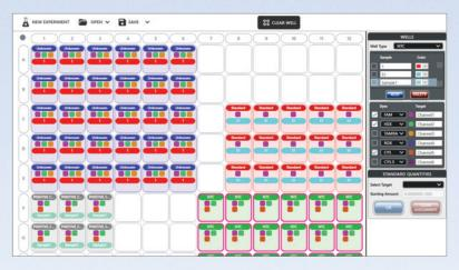
Quickly set up and confirm plate layout. Each well is color coded by sample type, biological replicate, and technical replicate. Well type and standard curve values are also easily visible.
